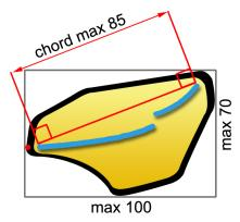
The side dams must be able to contain a square area of minimum 40 mm width and a minimum height of 50 mm to place the car identification numbers (downloaded from IFMAR website), from 1 to 12 at both external sides of side dams.
