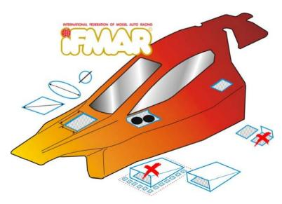
If no "marked" air scoops/vents are designed in the original mould to assist airflow to the motor or ESC, then material may be removed to a maximum of 10 mm in any given direction within a maximum square area of size 30 mm x 30 mm, in two places only. Windows are not allowed to be removed or include holes, other than for the purpose of the antenna.
